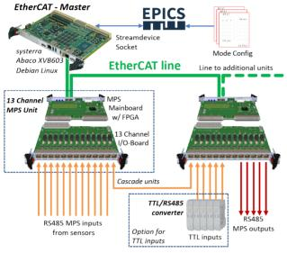
Figure 8: Machine Protection System core components.
