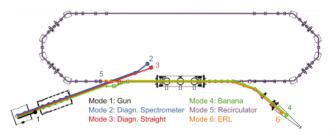
Figure 1: Basic bERLinPro layout and planned operation modes.
