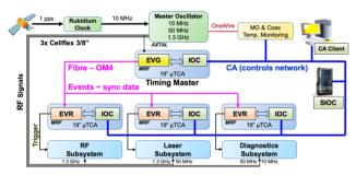
Figure 3: Schematic of timing system with master oscillator, RF distribution and trigger distribution system.
