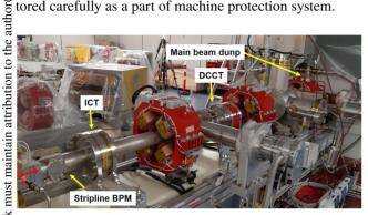
Figure 5: Stripline BPM, ICT, DCCT installed in main beamdump line.
