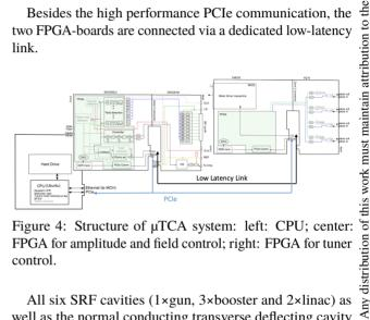
Figure 4: Structure of µTCA system: left: CPU; center: FPGA for amplitude and field control; right: FPGA for tuner control.
