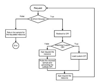
Figure 4: The flowchart shows the CFET returns different result based on the request when access the resources and generate suitable HMIs based on the resources.
