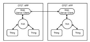
Figure 3: The block diagram of the CFET and the dataflow when accessing resources between components.
