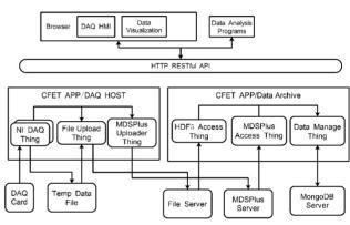
Figure 5: The block diagram of the ECEI DAQ system. The arrows are the data flows. The data flow inside and between CFET APP is handled by the CFET hub.
