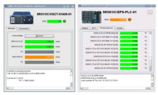
Figure 2: Different panels automatically generated for different types of devices in TANGO.
