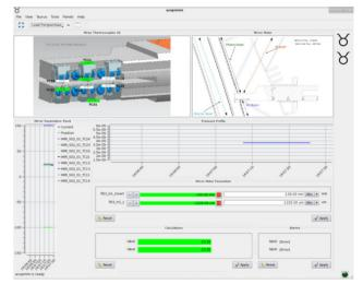
Figure 1: Taurus [4] GUI created by ALBA operators to manage the insertion/extraction of an infrared mirror.
