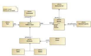
Figure 1: TANGO-Controls simplified data model.
