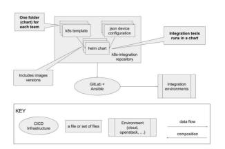
Figure 4: K8s Integration repository module view.
