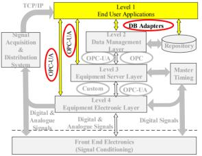
Figure 2: CNAO Control System Layered Architecture.
