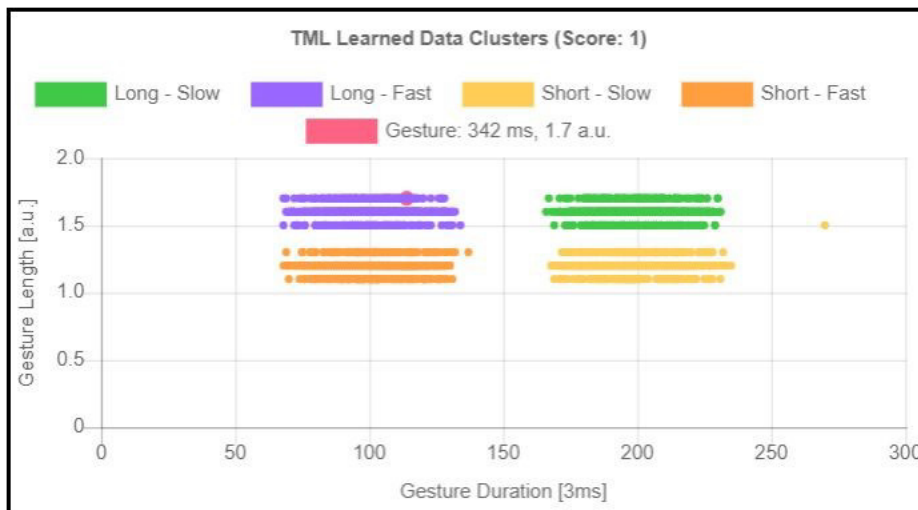
Figure 2: Predicted gesture duration / length and learned data clusters. The predicted movement (red dot) is classified as a Long-Fast movement.
