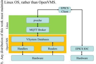
Figure 1: Overview of Vsystem/EPICS bridge pvecho (left), and ordinary IOC (right).
