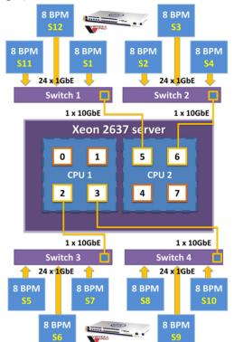
Figure 3: Block diagram of the DPDK test setup in the global orbit feedback system.
