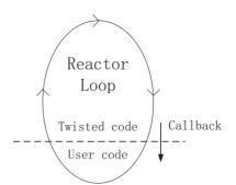
Figure 4: Callback pattern in the Twisted framework.
