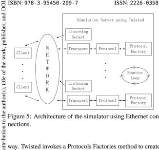
Figure 5: Architecture of the simulator using Ethernet connections.
