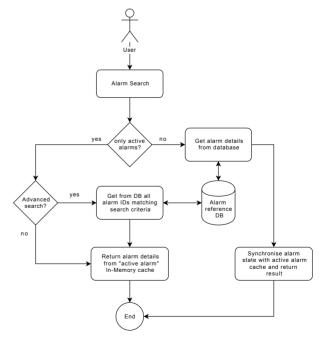
Figure 2: Workflow for optimising speed of search results.
