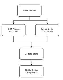
Figure 3: Front-end Workflow.
