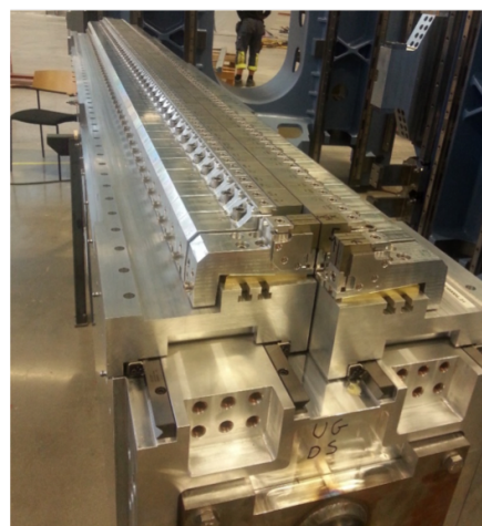
Figure 2: Each EPU girder has two subgirders that host the magnet arrays and can move relative to each other and to the subgirders in the other girder. Together they determine the polarization of the light.
