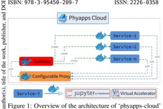
Figure 1: Overview of the architecture of 'phyapps-cloud' the platform. All the apps are Docker containers, managed by Docker Swarm. The users can connect through Configurable Proxy to the gateway, where all the private computing services (Service-i) could be spawned.
