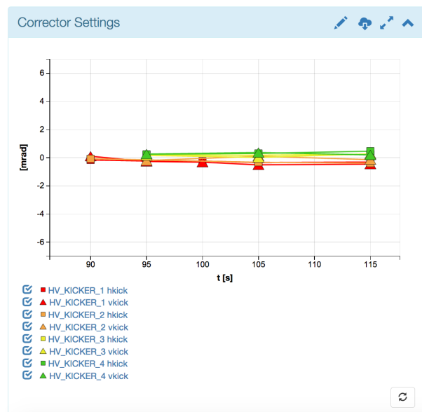
Figure 7: Screenshot of the corrector settings diagnostic showing the corrector settings as a function of time during an optimization.
