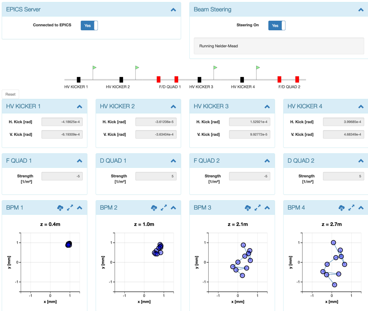
Figure 5: Screenshot of the accelerator controls landing page during a Nelder-Mead optimization.
