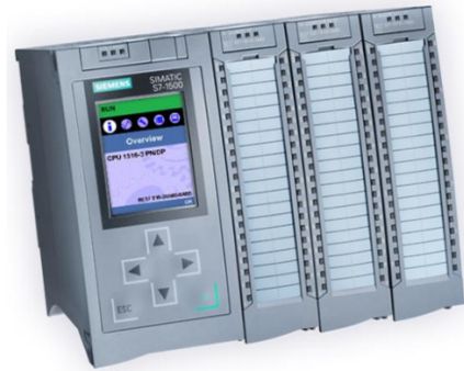
Figure 6: Siemens 1516-3 PN/DP CPU and cards.
