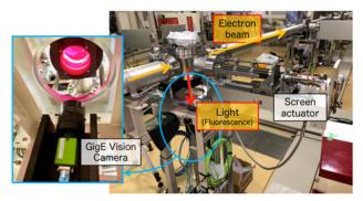
Figure 5: Screen monitor for SSBT.
