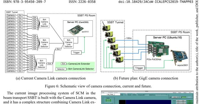
(a) Current Camera Link camera connection
