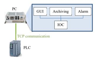
Figure 1: Small experiment architecture based on PLC.
