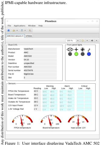
Figure 1: User interface displaying VadaTech AMC 502 information obtained from IPMI, including FRU, sensors 2019). and PICMG lights.
