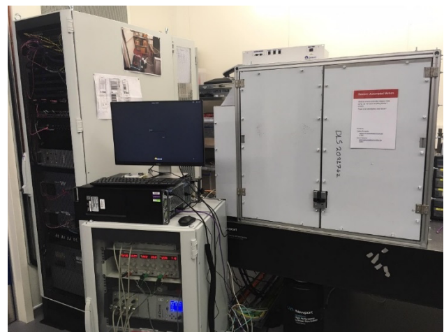
Figure 1: P99 optical development rig in the precision metrology laboratory, complete with main and small testing rack, opaque enclosure and beamline workstation.
