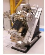
Figure 1: Wire Scanner at SLAC [1].
