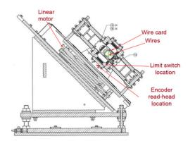
Figure 2: Wire scanner schematics showing the motor, encoder and limit switches.
