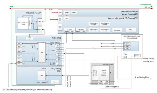
Figure 3: Controls System Architecture of Fast Wire Scanner at SLAC.
