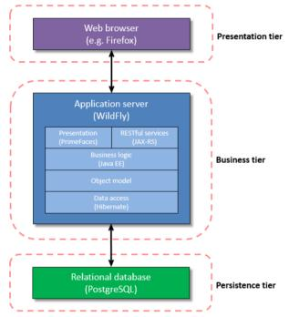
Figure 2: Architecture of the Cable Database.
