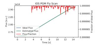
Figure 7: The estimated ideal flux and fractional deviation from ideal based on the monochromator following error.
