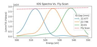
Figure 5: A comparison of the flux of the stationary state spectra at different gaps to the ideal flux from synchronized ID-monochromator fly scan motion.
