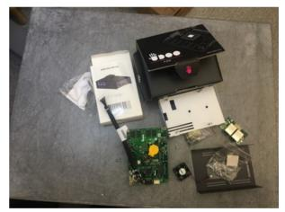
Figure 1: Unassembled hardware: UDOO Ultra board, two 1Gb Ethernet daughter card, metal case, cooling fan.
