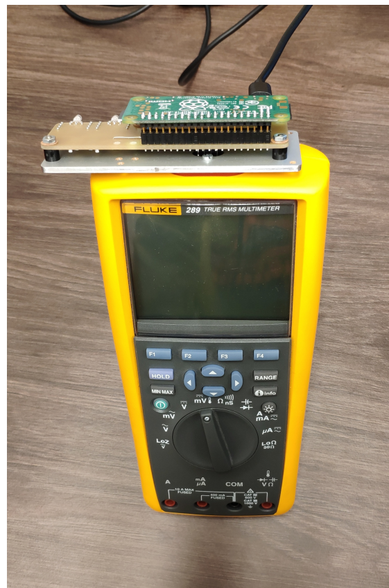
Figure 1: Holding plate with Pi Zero.
