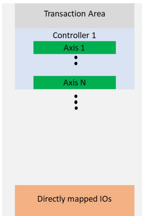
Figure 7: Layout of the PROFINET/BUS IO areas.
