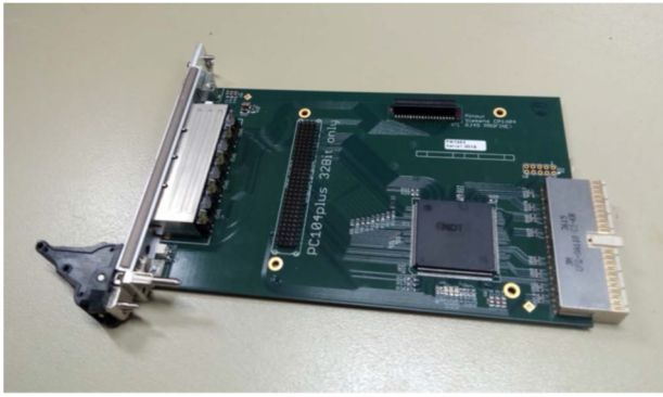
Figure 5: Photo of the new CompactPCI carrier for PC104+.
