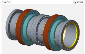
Figure 2: Schematic of two current transformers.
