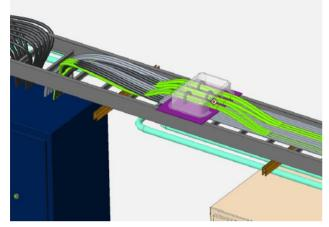
Figure 1: Schematic picture of the DCCT measurement of dipole magnet current.
