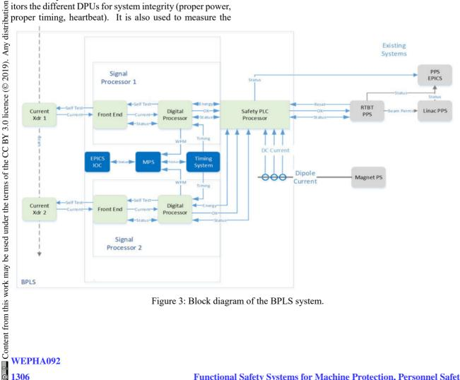
Figure 3: Block diagram of the BPLS system.
