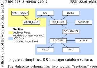
Figure 2: Simplified IOC manager database schema.
