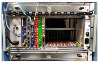
Figure 1: A µTCA crate with MCH, CPU, event receiver, Pico8, BPM and BCM cards.
