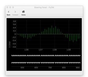
Figure 1: Linac Steering Widget in PyDM. The beam's transverse position (in the X or Y axis, depending on the panel being used) is plotted as a green bar. Below the plot of beam position measurements, increment/decrement controls for each corrector magnet are displayed. By clicking and dragging the plot, the user can pan the view to see different areas. Zooming in and out is possible by scrolling with the mouse wheel or trackpad.
