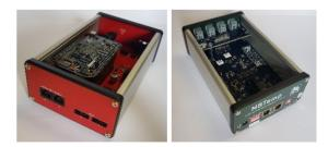
Figure 5: Multi-purpose counting system unit and MBTemp, which are being installed on Sirius accelerators.
