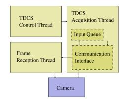
Figure 2: How the communication interface receives frames from the camera (solid lines), and passes commands and configuration changes to the camera (dashed lines).
