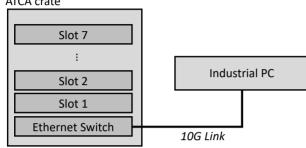
Figure 2: SMuRF system block diagram.
