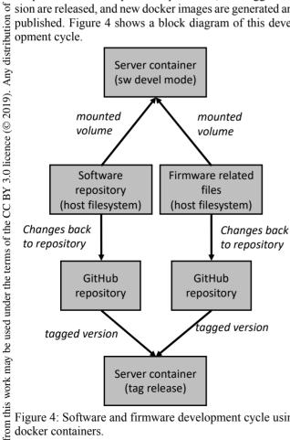
Figure 4: Software and firmware development cycle using docker containers.
