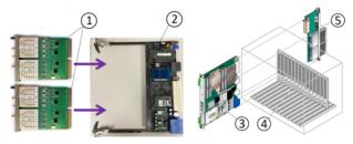
Figure 1: SLAC common platform hardware. 1) AMC daughter cards, 2) carrier card, 3) assembly of a carrier card with AMC daughter cards, 4) ATCA crate, 5) RTM card.
