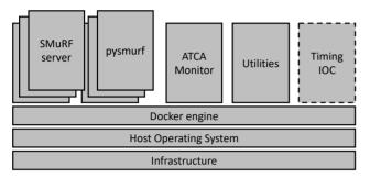
Figure 3: SMuRF application running in docker containers. The "Timing IOC" container is present only in some particular deployments.
