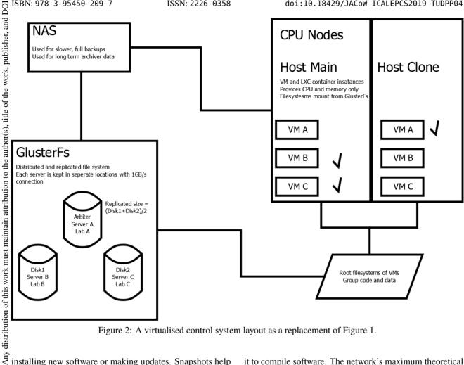
Figure 2: A virtualised control system layout as a replacement of Figure 1.
