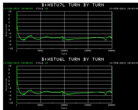
Turn-by-turn position measurement ACNET console display from Fermilab Booster
