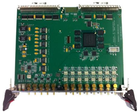
Accelerator Division / Instrumentation Department FPGA-based VME Digitizer Module
