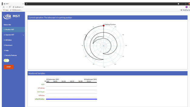
Figure 6: Screenshot of the browser-based GUI for monitoring and control of the MST structure. The black line illustrates the trajectory of the telescope pointing direction in azimuth and elevation.
