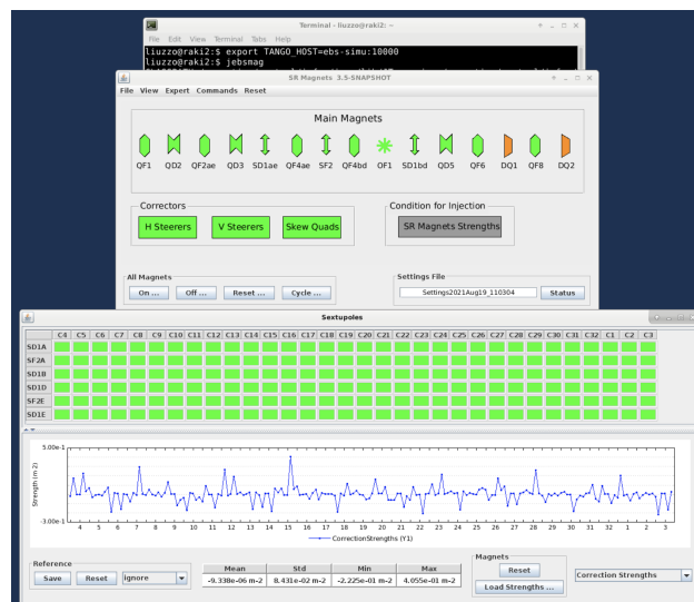
Figure 4: Application for the control of the individual magnets in strengths. Top, the main panel with family tuning, bottom, a view of the sextupole magnets.
