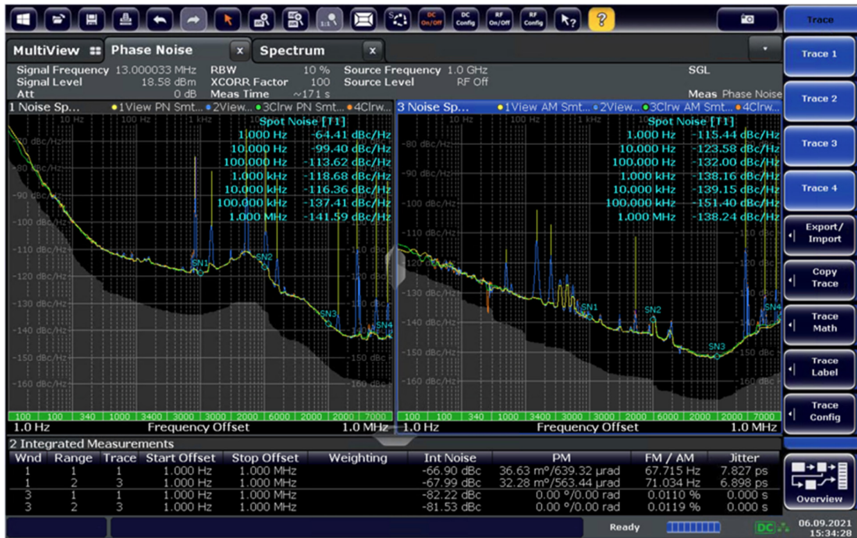
Figure 4: Output performance of a UNIV-LVPECL-DLY output module.
