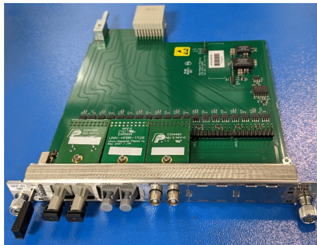
Figure 1: Micro Research Finland timing receiver rear transition module equipped with universal output modules.
