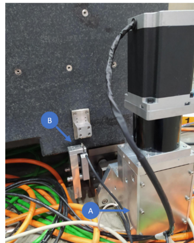
Figure 2: Leveller actuator (A) and feedback encoder (B).
