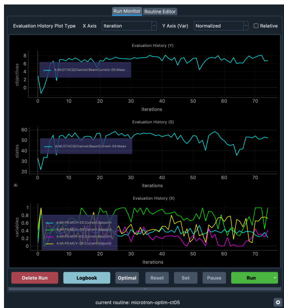
Figure 3: Screenshot of the Badger run monitor during microtron tuning. In the top panel, the objective progress is plotted. Additional observations (states) are monitored in the middle. The bottom panel shows the actuator values.
