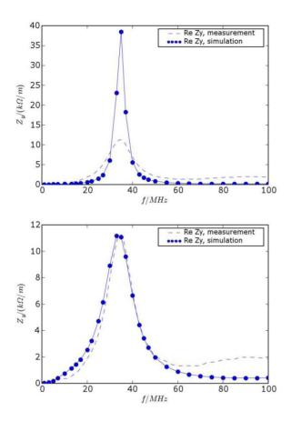
Figure 3:  $Z_y$  vs. frequency for the case  $Z_{ext} = \infty$ . The dotted line follows from simulation and dashed line from experimental measurements[4, 5].
