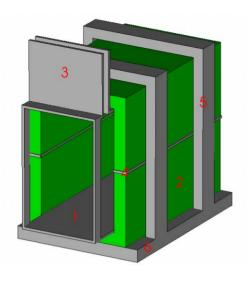
Figure 1: Schematic view of the SNS kicker where it is possible to observe the busbar (1), the ferrite (2), the end-plates of the busbar (3), the strips (4), a frame (5) and a base (6).
