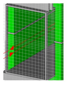
Figure 2: Schematic view of the SNS kicker where it is possible to observe the position and direction of the dipolar current.
