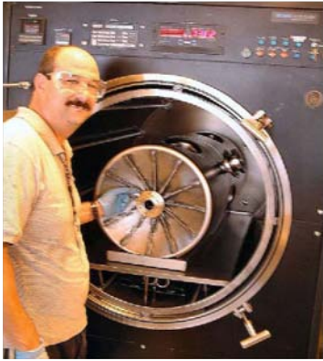
Figure 5. A 3D CAD model and a photograph of a superconducting triple-spoke resonator developed for the RIA driver linac.
