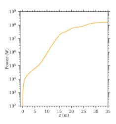
Figure 5: FEL radiation growth along the undulator length.
