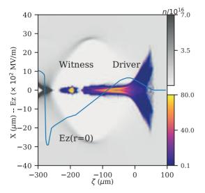
Figure 3: Bunch and background density colormaps after 5 mm within the plasma. The bunch density is plotted with a *plasma* colormap, while the background is plotted with a grey colormap. The longitudinal accelerating electric field, on axis, is over-imposed with a solid blue line. For scale purposes and for sake of clarity the Ez is plotted in hundreds of MV/m.
