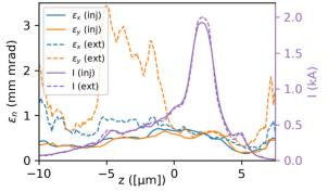
Figure 4: Slice analysis for the witness bunch at plasma input, dashed color, and at plasma exits, solid color.
