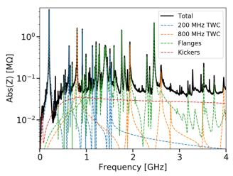
Figure 1: Longitudinal impedance model for the present configuration of the SPS. The contributions from the RF cavities, the vacuum flanges and the kicker magnets are also shown separatly [2, 16, 17].
