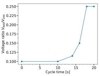
Figure 10: Optimised voltage ratio r between the two SPS RF systems during acceleration cycle for the LHC proton beam.
