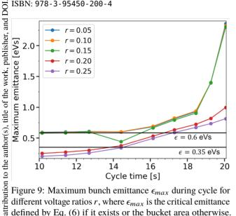
Figure 9: Maximum bunch emittance  $\epsilon_{max}$  during cycle for different voltage ratios r, where  $\epsilon_{max}$  is the critical emittance defined by Eq. (6) if it exists or the bucket area otherwise. The two horizontal lines show the nominal emittances at flat bottom (0.35 eVs) and at flat top (0.6 eVs).
