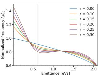
Figure 2: Synchrotron frequency distribution for the double RF system (n = 4) in BSM at SPS flat top as a function of the single particle emittance. For different values of the voltage ratio r, the frequencies are normalized by the synchrotron frequency in the bunch center computed for r = 0. The 200 MHz voltage is  $V_{200} = 7$  MV. The vertical black line indicates the nominal bunch emittance at flat top (0.6 eVs).
