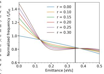
Figure 5: Normalised synchrotron frequency distribution for the double RF system in BSM at SPS flat bottom, as a function of the emittance for different value of the voltage ratio r. The 200 MHz voltage is  $V_{200} = 4.5$  MV. The vertical black line indicates the nominal bunch emittance of 0.35 eVs.
