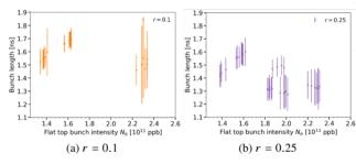
Figure 3: Average bunch length at flat top measured for batches of 12 bunches with nominal emittance (0.35 eVs). The error bars represent the maximum and minimum bunch length measured along the batch. The cases r = 0.1 (a) and r = 0.25 (b), kept during whole cycle, are presented. The 200 MHz voltage at flat top is 7 MV and feedback and feedforward were activated during whole cycle.
