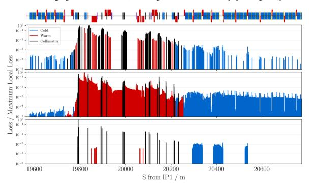
Figure 8: Loss map comparison, zoomed to IR7 where the betatron collimation is located, between beam loss monitor signal (top), BDSIM energy deposition (middle), and SixTrack losses (bottom). Each is normalised to the corresponding peak in IR7. Cold, warm, and collimator losses are encoded to highlight the various features, and a diagram of the machine is displayed along the top.
