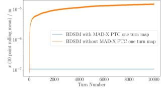
Figure 2: BDSIM long term tracking comparison for a reference particle. The transverse position x is recorded at the end of each turn for 10,000 turns with and without the use of a one turn map to correct the particle's trajectory.
