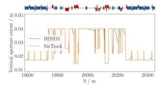
Figure 4: A comparison of the vertical aperture extents between BDSIM and SixTrack. The difference between the two shown is an artefact of the way apertures are described in BDSIM. A BDSIM does not have an aperture, but instead an *opening*, whereas the aperture is defined throughout for SixTrack, even where apertures are located.
