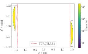
Figure 5: Primary distribution with collimator jaws marked. The primary distribution is shown zoomed inset as the region in phase space is extremely small.
