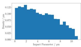
Figure 6: Probability density for the impact parameters on the horizontal collimator in IR7.
