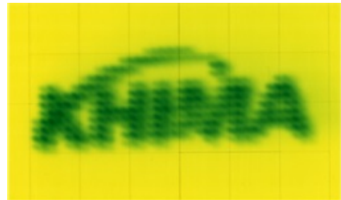
Figure 8: The obtained GaF film image obtained by using the prototype active scanning system.
