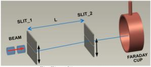
slit-slit emittance scanner
