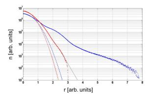
Figure 4: A phase space density plot for beam distributions measured in SNS 2.5MeV MEBT (red line) and 1GeV HEBT (red line).
