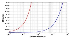
Figure 3: Dependence of the RMS size (blue line) and of the kurtosis (red line) on the halo amplitude for the profile of Fig. 2.
