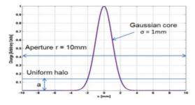
Figure 2: A test beam profile consisting of a Gaussian core and a uniform halo.
