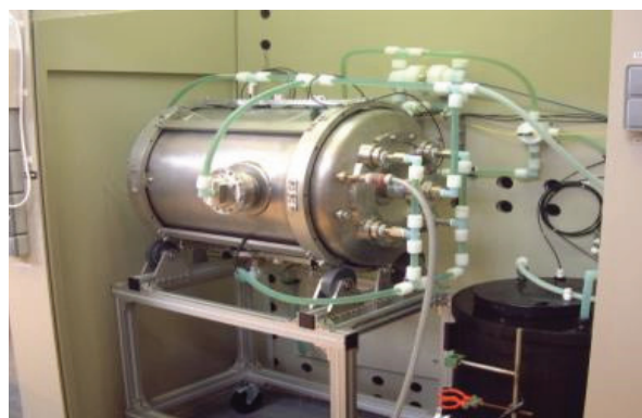
Figure 9: A spoke cavity under chemical etching at INO-CNRS at the SupraTech facility. The complete spoke cryomodules with cavities are designed and built by IPNO-CNRS. All three prototype double spoke cavities performed well above specifications in a vertical cryostat test. Picture courtesy of IPNO-CNRS.
