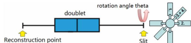
Figure 2: To obtain the beam matrix  $C$  at the reconstruction point all four emittance values are measured using ROSE behind a magnetic doublet.
