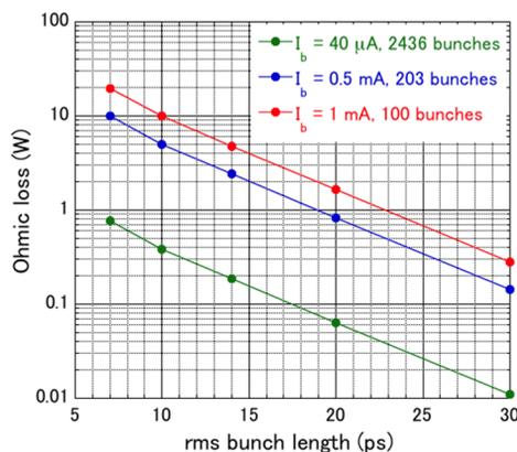
Figure 3: Calculated heat input to the BPM head for the total beam current of 100mA with bunch currents of 0.04 mA (green), 0.5 mA (blue) and 1 mA (red), respectively, as functions of the bunch length.
