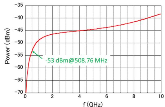
Figure 2: Calculated power spectrum of the button BPM signal from a 100 pC bunch with 10 MHz bandwidth.
