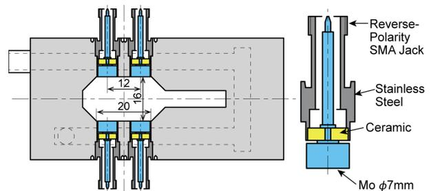
Figure 1: Schematic drawings of the cross-sections of the BPM head (left) and the button electrode (right).
