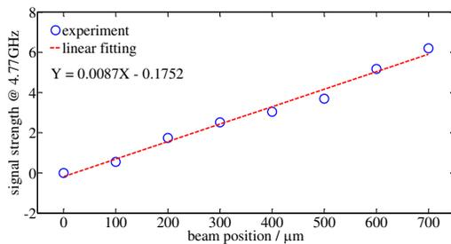
Figure 5: Linear relation between the beam position and the amplitude of the  $TM_{010}$  mode.
