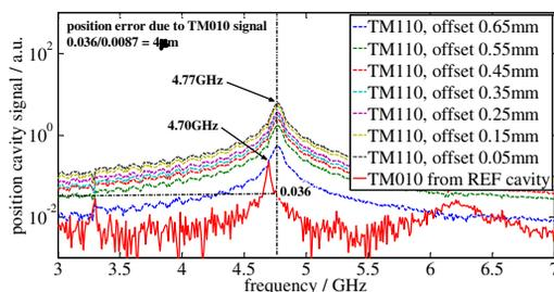
Figure 6: Amplitudes of the  $TM_{110}$  mode of the position cavity and the disturbance mode from the  $TM_{010}$  mode of the reference cavity.
