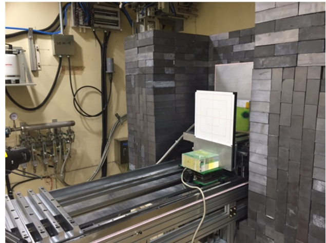
Figure 4: Experimental setup of the beam profile measurement by using 2D ionization chamber array.
