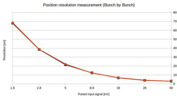
Figure 10: Position rms (30 dB dynamic range / FWHM=100ns).
